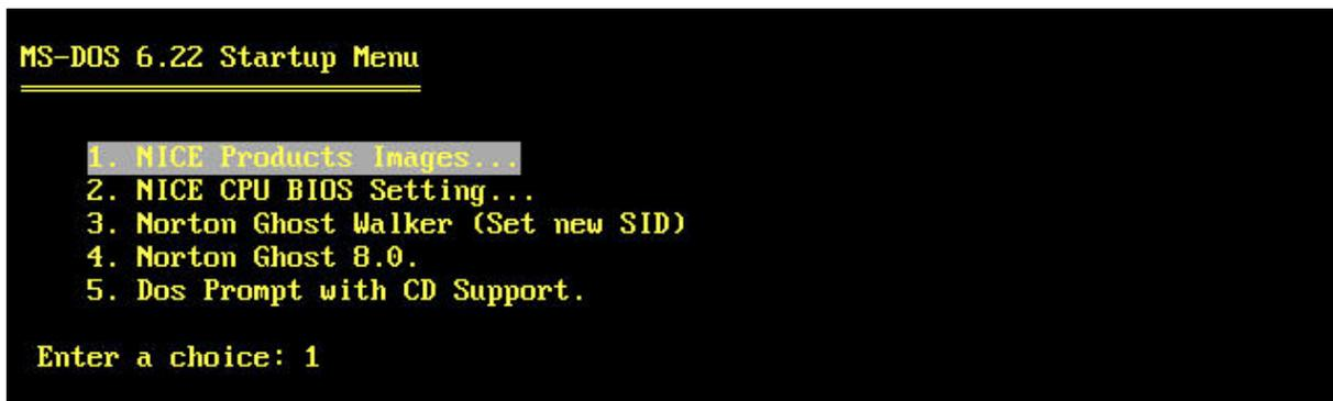
2. From the MS-DOS 6.22 Startup Menu now select machine type (1 – NiceLog PCI / 2 - ICU / 3 – NiceLog ISA 8.9) and press Enter.
